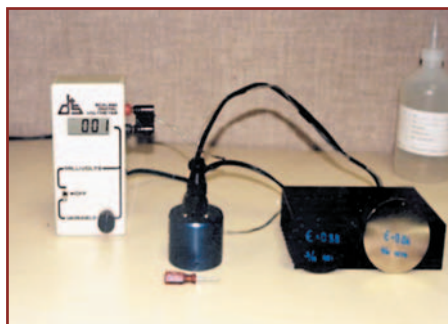
Photo 2: This apparatus is used with the ASTM C-1471 emittance test protocol.
