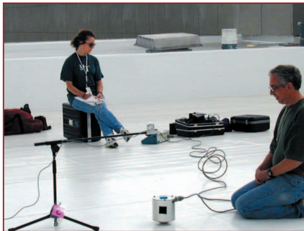
Photo 1: The microphone stand attached to a small meter (off camera) measures reflectance. The instrument which appears to be a gallon paint can attached by wire to a small suitcase is performing the D&S test.
